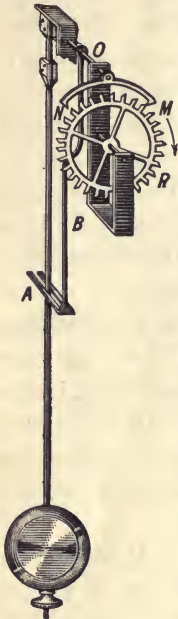
FIG. 44. — Escapement and Pendulum of a Clock.
